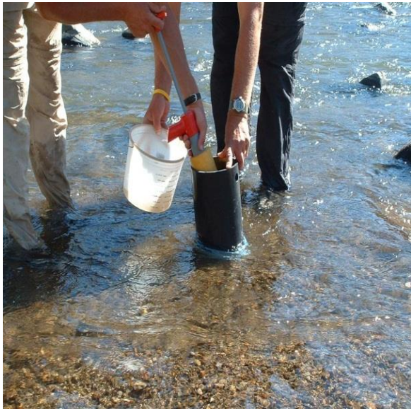
Figure 3. Pump-core sampling device, using hand-operated bilge pump to remove contents of isolated core area (left) to measure fine sediment volume (right), and associated benthic macroinvertebrates.
