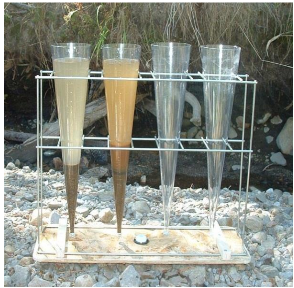
Figure 3. Pump-core sampling device, using hand-operated bilge pump to remove contents of isolated core area (left) to measure fine sediment volume (right), and associated benthic macroinvertebrates.
